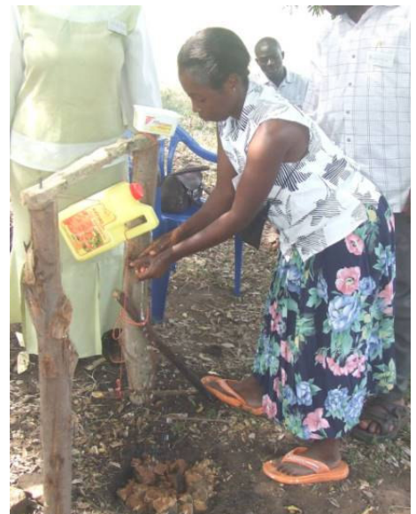
The tip tap is made from an old plastic container, and is operated by the foot.
